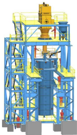
ENDURON® Optimil vertical stirred mill (VSM)
