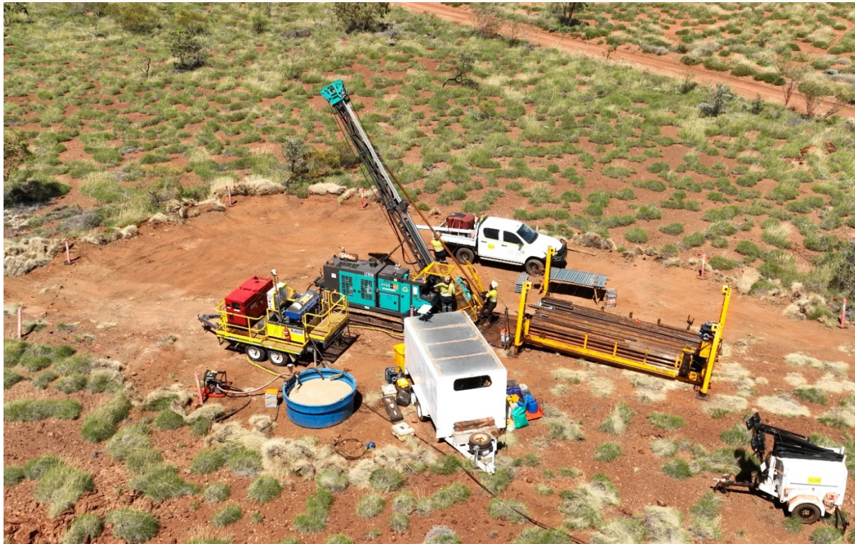
Photo 1. Diamond drill rig site at Elizabeth Hill. Drilling was completed in early July, after which the drill rig and crew were demobilised.
