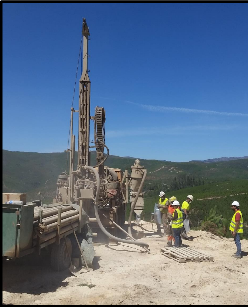
Figure 4. RC drilling at Grandao
